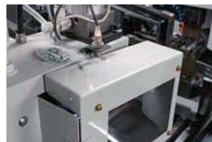
切削部カバー (安全装置 開時運転停止) Cutting section cover (Safety device: Operation stops when open)
